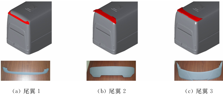
图 2 3 种尾翼方案的造型和安装位置 Fig. 2 Designs and installation positions of three rear spoiler
