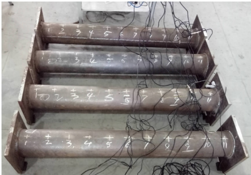
图 5 钢管混凝土柱试件及测点布置 Fig. 5 CFSTC test pieces and layout of measuring points
