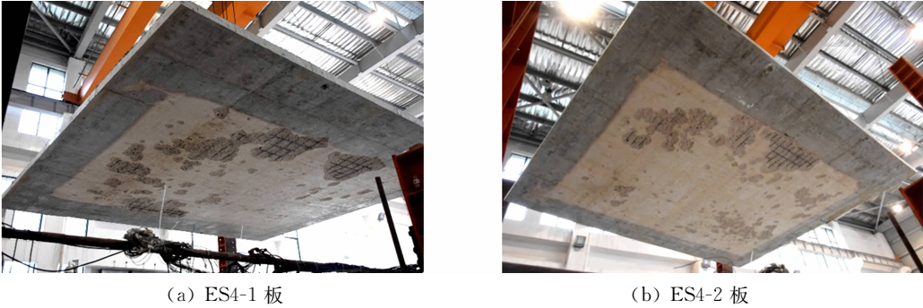
图 9 双向板板底爆裂实景图 Fig. 9 Picture of bottom burst of two-way slab
