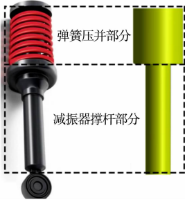
图 1 减振器三维变截面圆柱模型示意图 Fig. 1 Schematic diagram of three-dimensional step cylinder model of shock absorber
