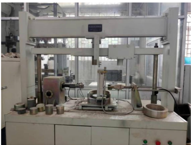
图 3 道路材料弹性模量、剪切强度测试仪 Fig. 3 Resilient modulus and shear strength test device of road material
