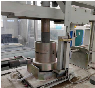
图 10 级配碎石混合料的抗压回弹模量试验仪器 Fig.10 Test instrument for compressive resilient modulus of graded crushed stone mixture
