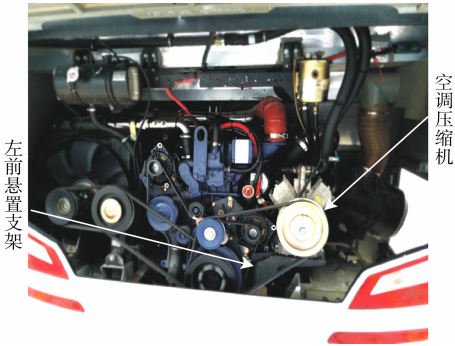
图 2 搭载空调支架实图 Fig. 2 Equipped with air conditioning bracket real map
