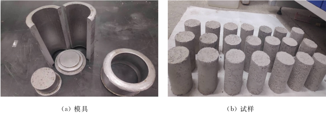
图 1 模具及试样 Fig. 1 Mold and sample
