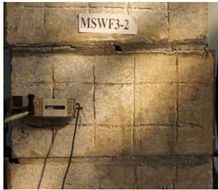
图 3 灰缝典型破坏形态 Fig. 3 Typical failure mode of mortar joint
