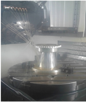
Fig. 18 Face milling of conical cycloid tooth
