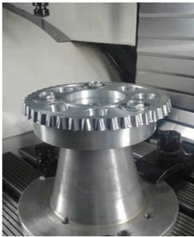
Fig. 19 Conical cycloid gear prototype after precision face milling
