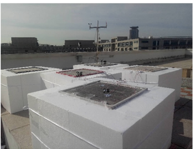
图 2 混凝土屋面实验小室布置 Fig. 2 Concrete roof experimental chamber arrangement
