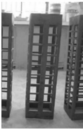
图 4 钢板笼试件 Fig. 4 Specimens of prefabricated steel cage
