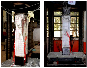
图 4 轴心受压破坏图 Fig. 4 Damage under axis compression
