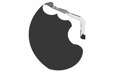
图 7 液压挖掘机工作装置作业范围 Fig. 7 Reachable range of working device of hydraulic excavator
