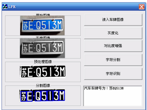
图 5 汽车车牌字符识别软件 Fig. 5 Vehicle license plate character recognition software
