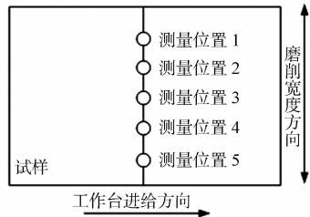
图 5 残余应力测量位置 Fig. 5 Residual stress measurement of ground surface
