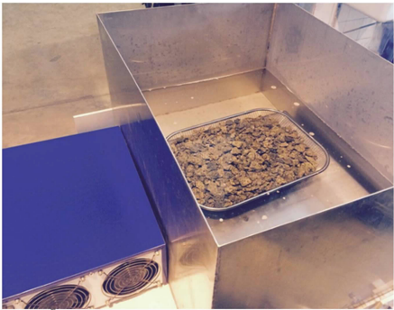
图 1 超声波促进麦饭石溶出装置图 Fig.1 Equipment diagram of ultrasonic promoting the digestion of elements from the medical stone
