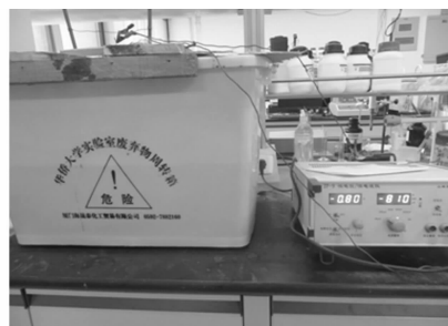
图 1 50 L 规模 Fe-P 电镀装置 Fig. 1 Plating Fe-P device of the scale of 50 L bath
