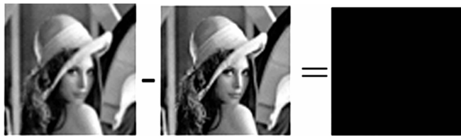
(a) g_1(x, y) (b) g_2(x, y) (c) DoG 边缘检测结果
