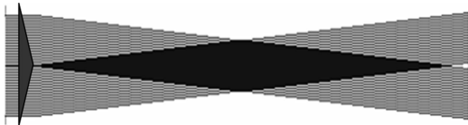
图 2 轴棱锥产生无衍射光的几何光线追迹 Fig. 2 Geometrical ray-tracing of non-diffraction beams generated by an axicon
