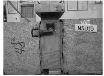
(c) II 型破坏(带连接件)
